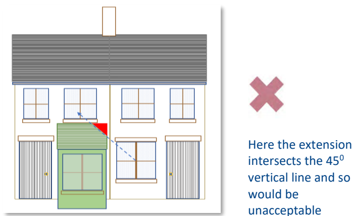
Figure 11: The 45° Rule diagram – front view
